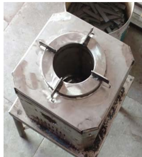
Fig. 6: Modified Cookstove along with Upper covering
