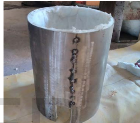
Fig. 3: Thermal Insulation of Combustion chamber
